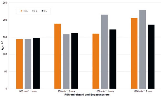
Fig. 2: k<sub>L</sub>a values for the Minifors 2 at 900 and 1200 min<sup>-1</sup> and 1 and 2 vvm.
