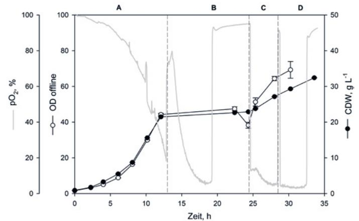
Fig. 4: Process overview of the batch/pulse method showing biomass growth on glucose (phase A, 0 to 13 h) and subsequent induction via MeOH pulses (phases B-D, 1% v/v).
