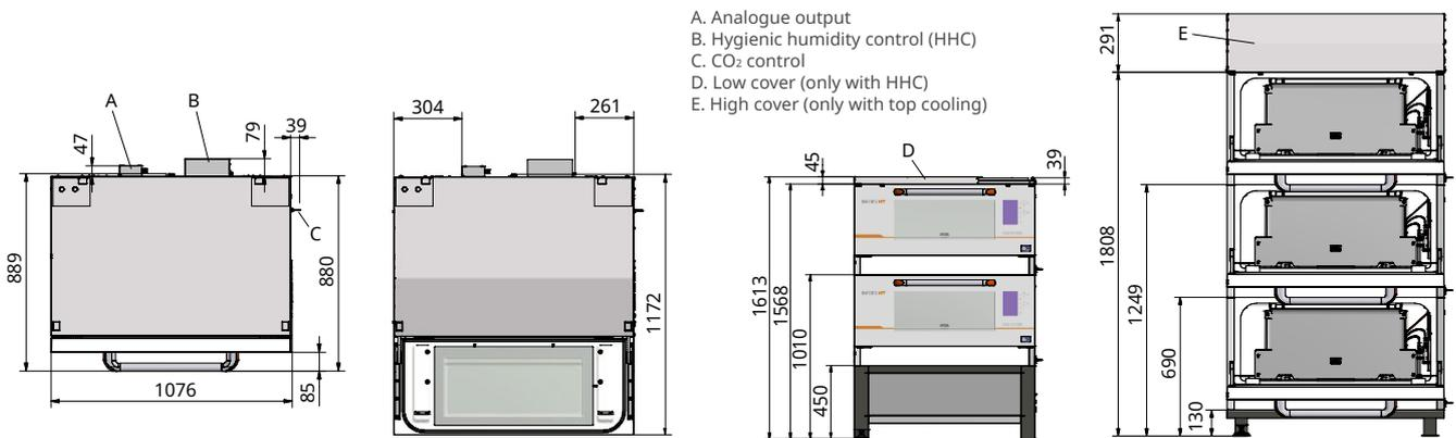
Note: The dimensions above only apply to the 230 V version. The heights of the bases of the 115 V version are slightly different (high base = 406 mm instead of 450 mm; low base = 140 mm instead of 130 mm).
